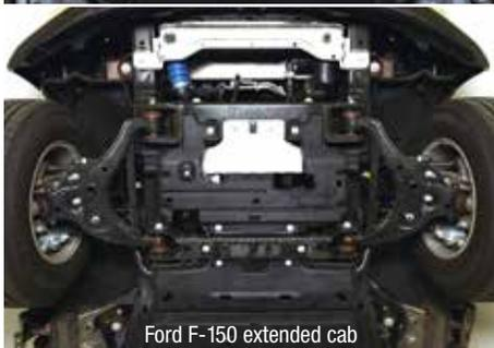
This undercarriage view of the crew cab (top) and extended cab shows where Ford beefed up the crew cab's front frame. IIHS painted the added elements red and yellow.
