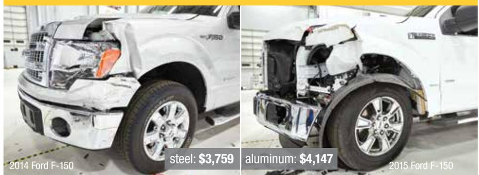
The aluminum F-150 took longer to repair than the steel pickup, pushing up the bill for the front test. Mechanics had to assemble wiring and other components before a new fender could go on.
